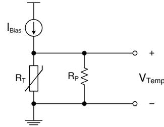
**Figure 8-4. Current Biasing Circuit With Non-Linear Thermistor**
