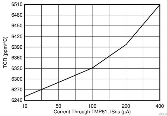
**Figure 6-3. TCR vs Sense Currents ( $I_{SNS}$ )**
