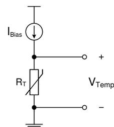
Figure 8-2. Current Biasing Circuit With Linear Thermistor
