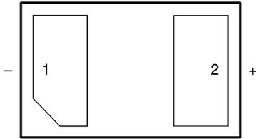
Figure 5-1. DEC Package 2-Pin X1SON Top View
