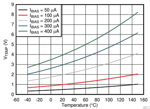
Figure 8-7. TMP61-Q1 Temperature Voltage With Varying Current Sources
