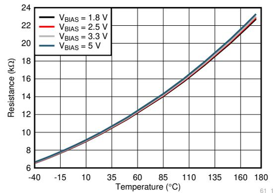
$R_{BIAS} = 10\text{ k}\Omega$  with  $\pm 0.01\%$  tolerance
