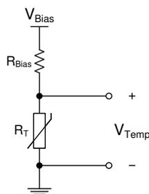
Figure 8-1. Voltage Biasing Circuit With Linear Thermistor
