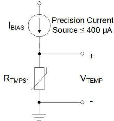
Figure 8-6. TMP61-Q1 Biasing Circuit With Current Source
