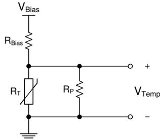
**Figure 8-3. Voltage Biasing Circuit With Non-Linear Thermistor**
