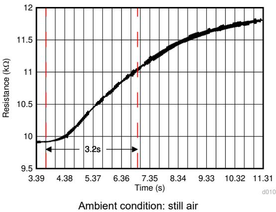
Figure 6-9. Thermal Response Time (DEC and DYA Package)
