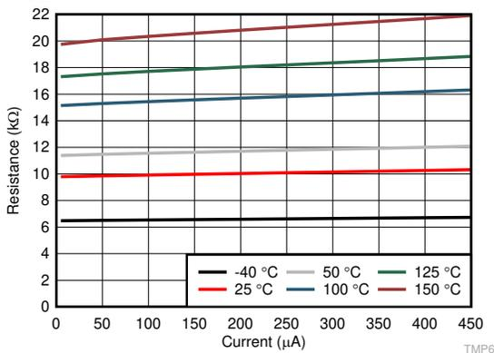
**Figure 6-5. Supply Dependence Resistance vs Bias Current**
