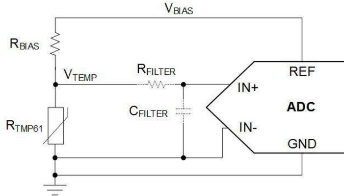
**Figure 8-5. TMP61-Q1 Voltage Divider With an ADC**
