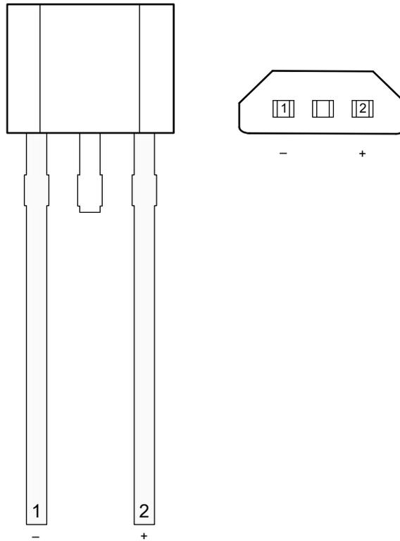
Front view is described as chamfers of TO-92S facing the user. Bottom view is described as pins coming out of the page.
